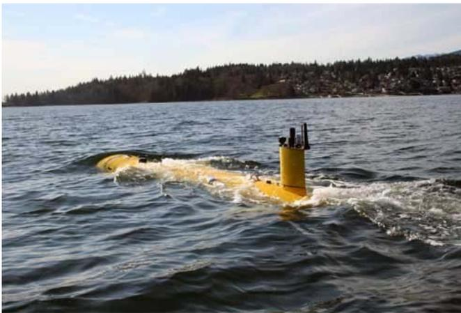
MARUM's new AUV, named SEAL, is rated to a depth of 5000 meters and has an endurance of 24 hours at a speed of 1.5m/s. This and a payload capability of 100kg provide the ability to conduct a wide variety of missions including seabed surveys or in the water column.
