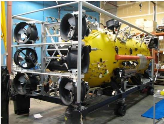
The PRMS Vehicle (PRM) is a remotely operated submersible whose payload is a pressure vessel capable of transporting 18 adults. The occupants of the pressure vessel can control their environmental conditions but cannot maneuver and navigate the vehicle. The PRM is piloted remotely from a surface Vessel of Opportunity (VOO), in a manner similar to a traditional ROV. ISE is a subcontractor to OceanWorks International Corporation who is the prime for the PRMS project.
