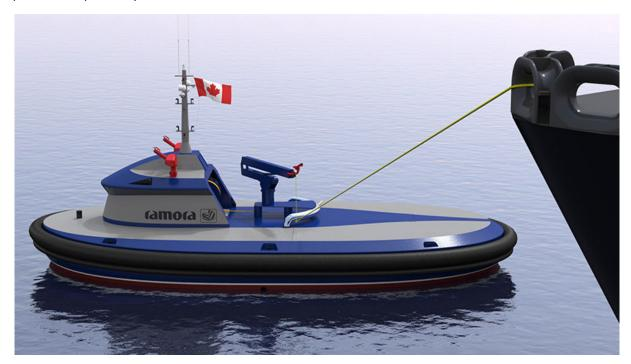
In keeping with Robert Allan Ltd.'s commitment to design top performing workboats, *RAmora* is fitted with Voith Schneider Propeller (VSP) drives arranged in a fore/aft configuration for exceptional omni-
