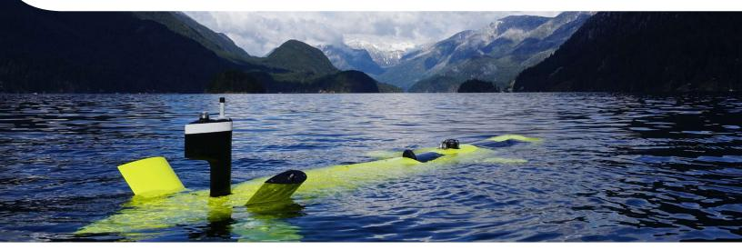
The ISE EXPLORER Autonomous Underwater Vehicle (AUV) collects **IHO compliant data** at a rate of **750 to 1100 km per week** of ship time with all sensors operating and is the most modular and maneuverable AUV in the world today. The modular design of the EXPLORER enables it to carry multiple payloads in its spacious, swappable, and customizable payload section.
