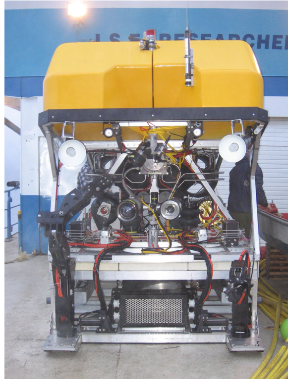
Hysub 130 with Science Sled Fitted with Sample Drawer
