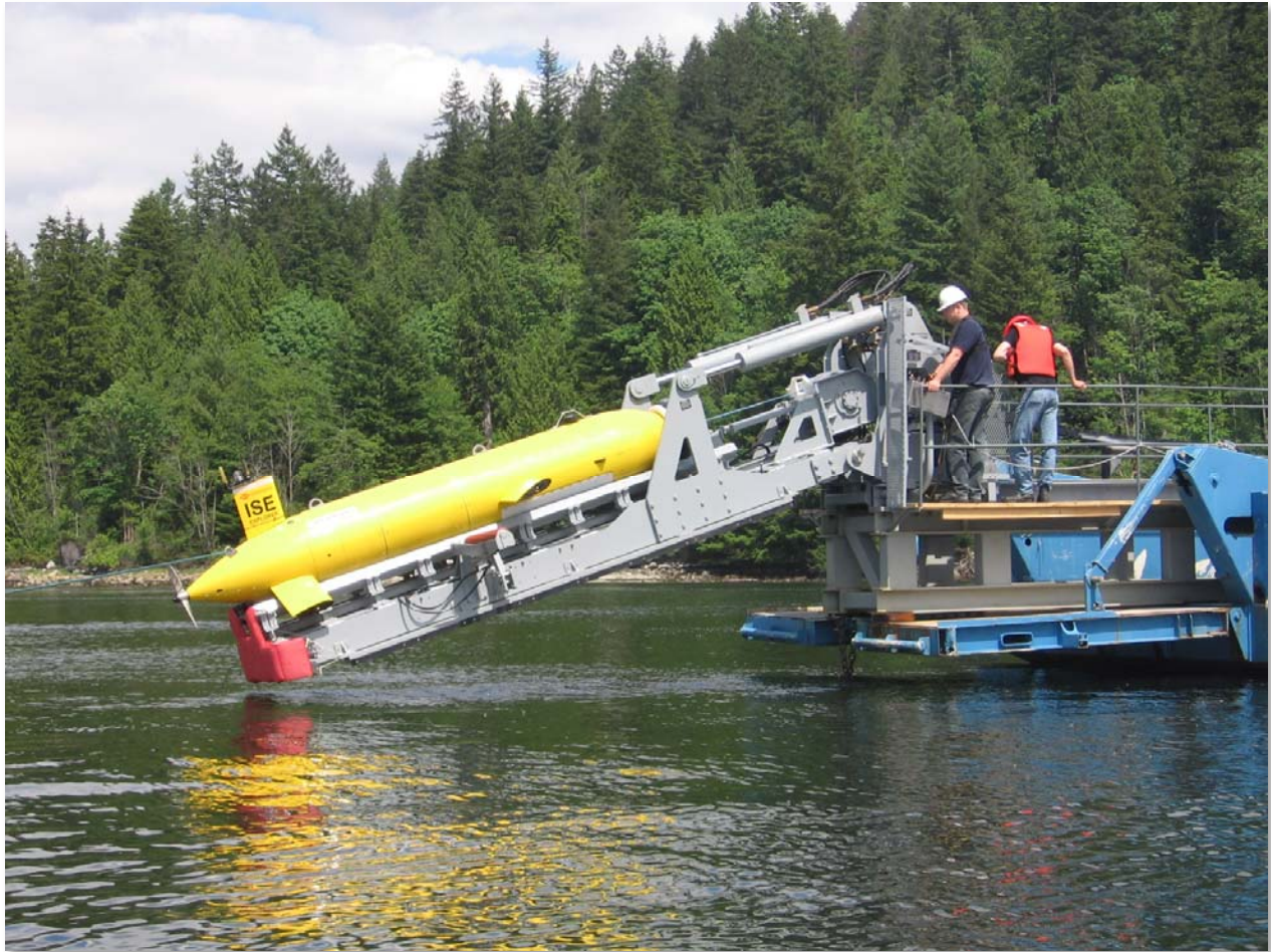
AUV with self-articulating ramp-based Launch and Recovery System (LARS)
