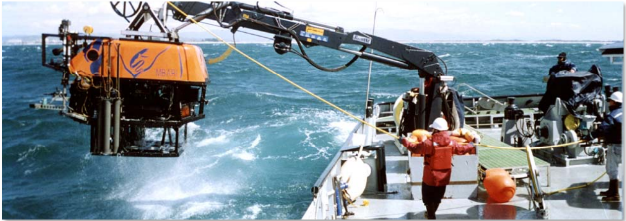
VENTANA ROV operated by Monterey Bay Aquarium Research Institute
