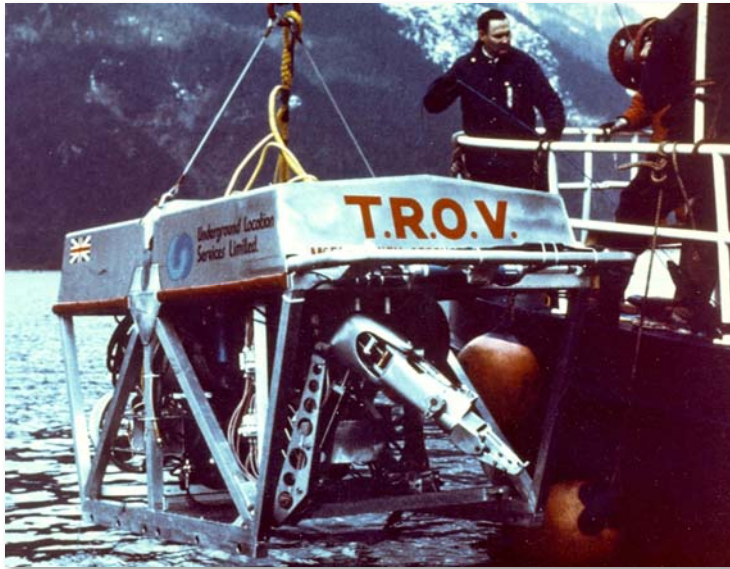
TROV (Tethered Remotely Operated Vehicle) One of the first ROVs developed by ISE in 1976
