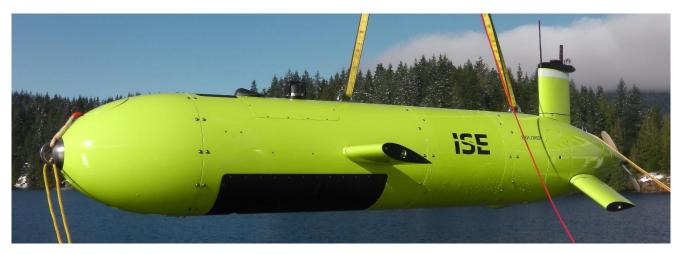
Port Coquitlam, BC - International Submarine Engineering Ltd. (ISE) announced today the sale of the latest ISE Explorer AUV to China Ocean Mineral Resource R&D Association (COMRA). This ISE Explorer AUV is the first rated for operations at 6000 m depth.
