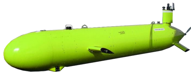
Explorer family of AUVs 3000 to 6000 m operational depths
