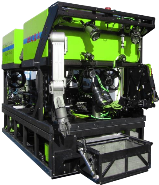
HYSYUB family of work-class ROVs 50 – 250 hp / 1000 – 6000 m depth ratings
